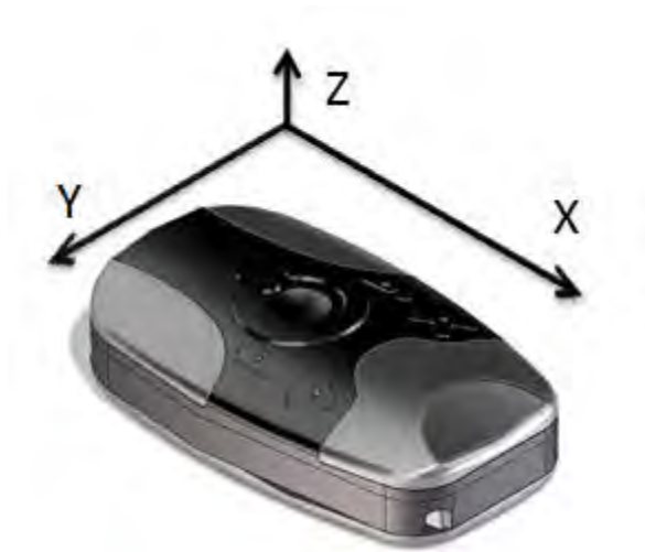
Figure 12 Accelerometer axis directions
