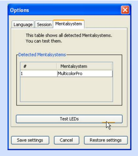
The file card "Mentalsystem" shows you all detected Digital Mentalsystems at your PC. You can test the LEDs if you click on "Test LEDs". The LEDs must flash if you test them. If you are not flashing there is a problem with the driver or the device is not connected, please read the chapter "In case of trouble".
